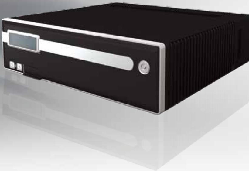
BP-500 is an high performance box PC that is designed with high flexibility and scalability. BP-500 POS features options of an Intel® Celeron®, Pentium® or Core i5 processor. This point of sale hardware is ideal for retail applications to optimize store operations. In addition, the rich I/O interface gives the terminal high expandability allowing it to grow with its environment.
